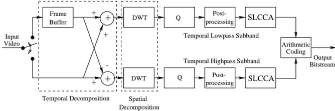
Fig. 2. Block diagram of 3D-SLCCA encoder.
